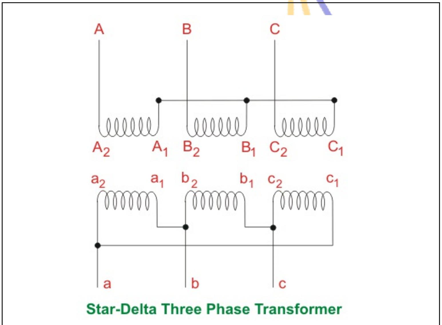
The delta connection in LV side is formed by connecting 1 suffixed terminals of each phase LV winding with 2 suffixed terminal of next
