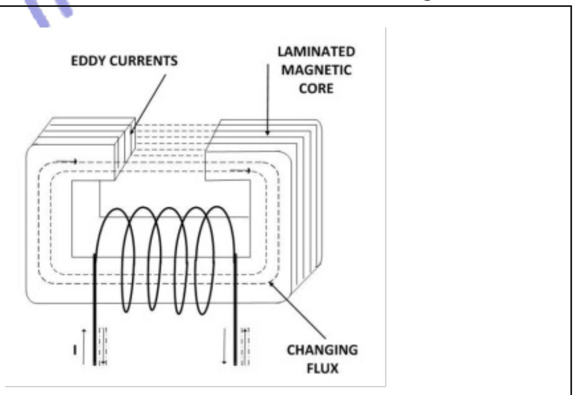
Eddy currents are undesirable since they heat up the core and dissipate electrical energy in the form of heat.
