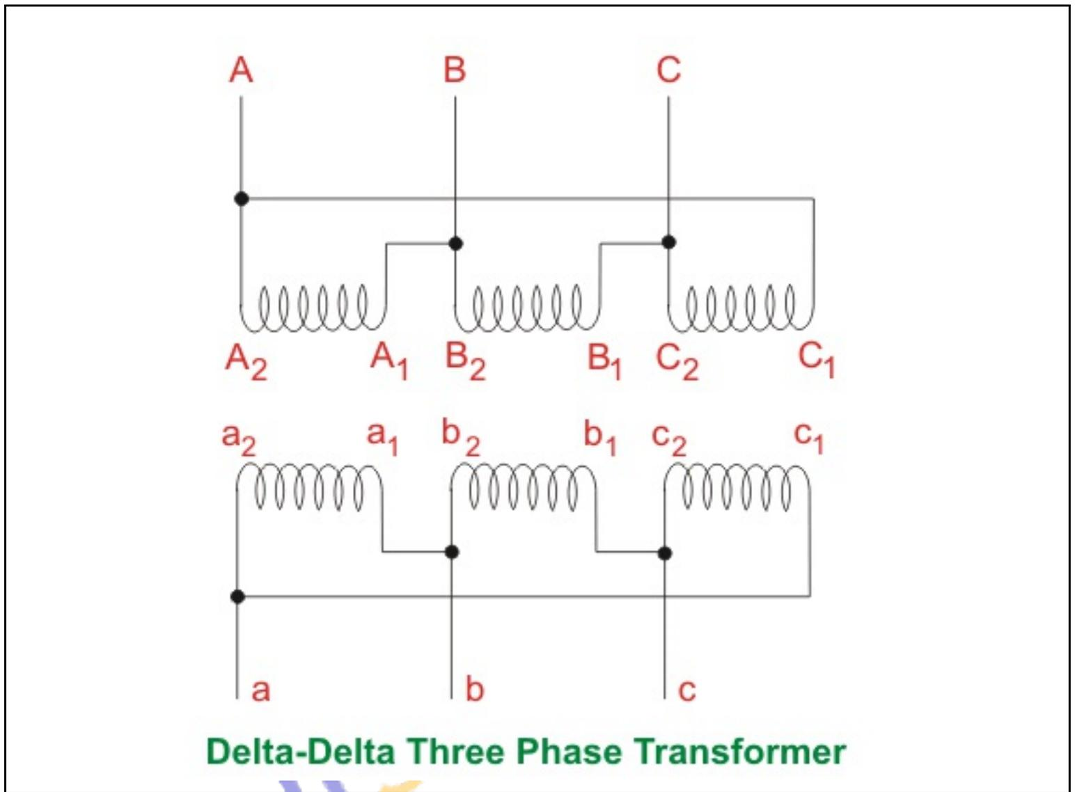
If primary is HV side, then A1 will be connected to B2, B1 will be connected to C2 and C1 will be connected to A2. Similarly in LV side 1 suffixed terminals of each phase winding will be connected with 2 suffixed terminals of next phase winding. That means, a1 will be connected to b2, b1 will be connected to c2 and c1 will be connected to a2.
