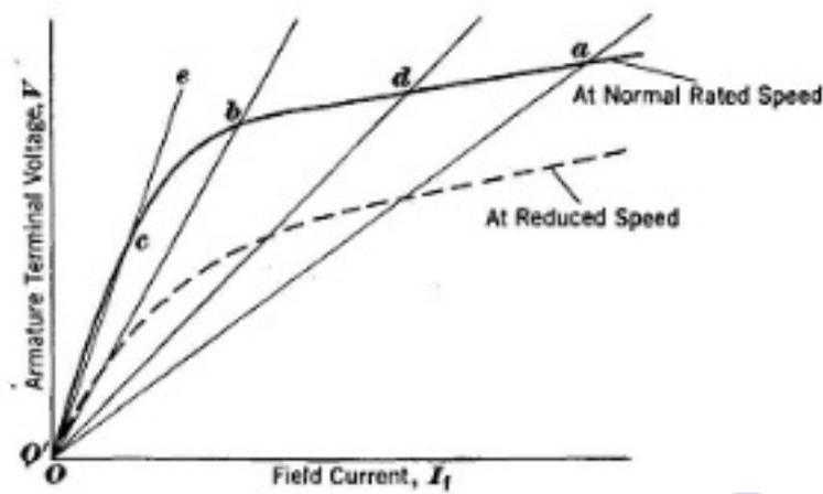
If the resistance is made so high that the slope of the resistance line, as  $Oe$ , is equal to or greater than that of the lower straight part of the magnetization curve, the voltage of the generator will collapse and will drop to the residual value  $O'$ . A generator may fail to build up for any of the following reasons:
