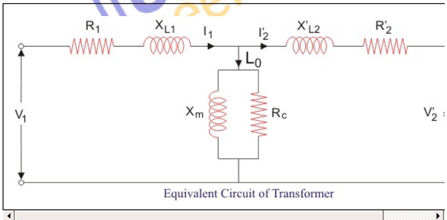
Let us define  $x\%$  be the percentage of full or rated load 'S' (VA) and let  $P_{cufl}$ (watts) be the full load copper loss and  $\cos\theta$  be the [power factor](#) of the load. Also, we defined  $P_i$  (watts) as core loss. As copper
