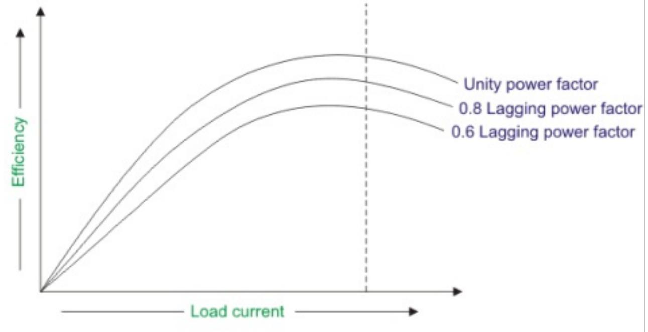
We can see from the figure that the maximum efficiency occurs at unity power factor. And the maximum efficiency occurs at the same loading irrespective of power factor of the load.
