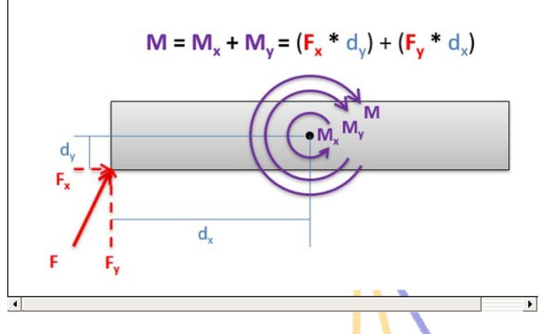
Breaking a force into components to solve for the overall moment
